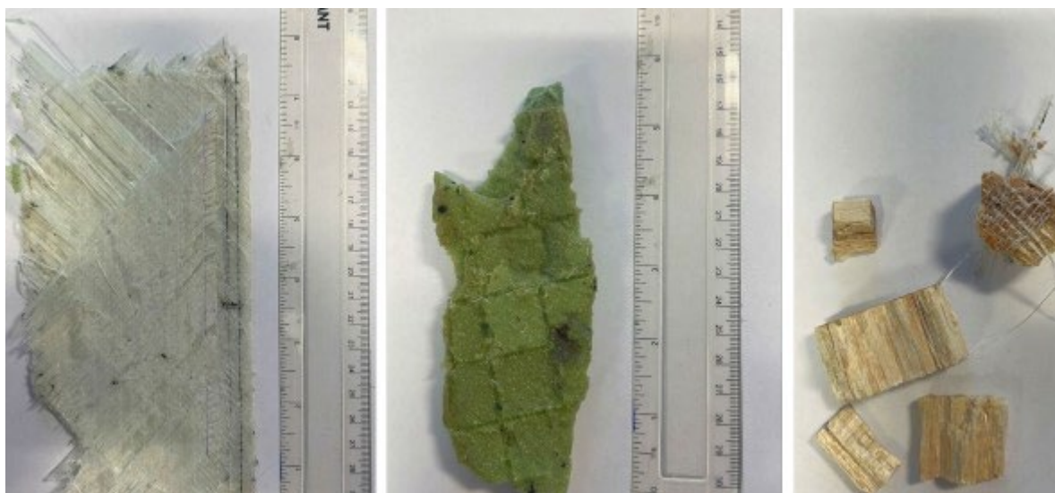
Debris has fractured off from one of the blades and will likely reach the shore. 16 17
