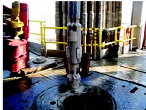
Figur 3.6 Borekrone. (TSS Energy AS)
