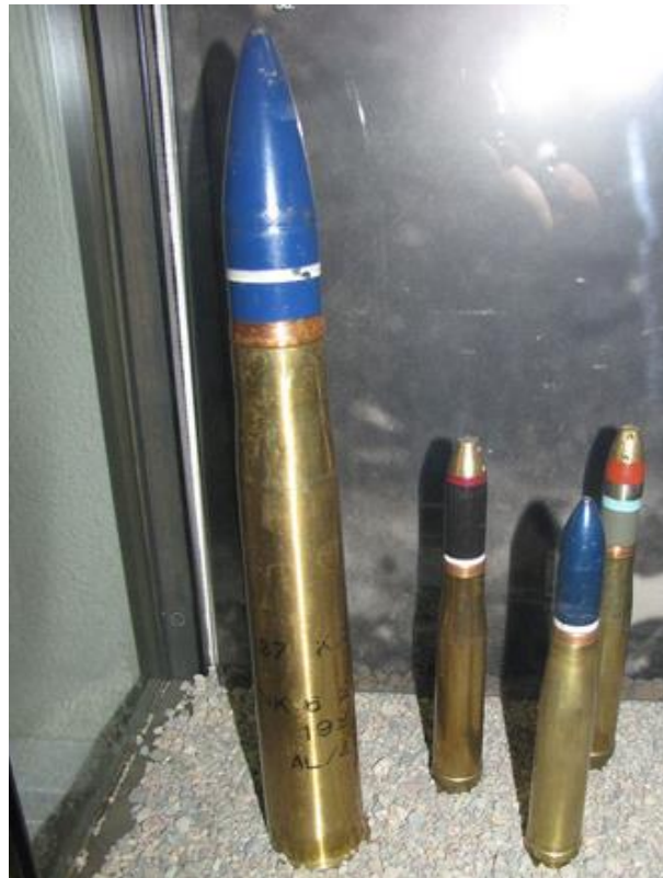
Figure: 37 mm and 20 mm rounds
