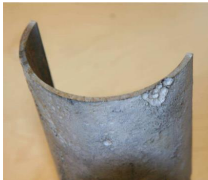
Figure: Shell segment of forged mercury container cut through area with maximum metal loss
