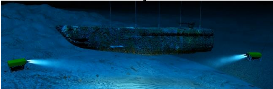
Figure: The ROVs monitor the process and send video to the control room of the salvage vessel
