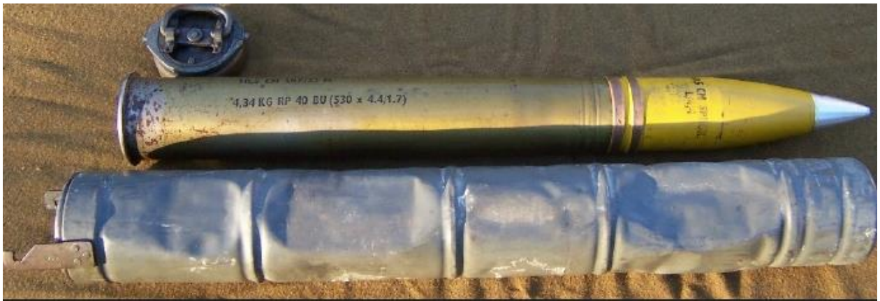
Figure: 10.5 cm SK C/32 round with steel container
