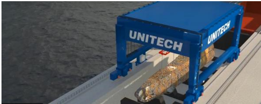
Figure: The U-864 wreckage parts are moved onto the dock bed
