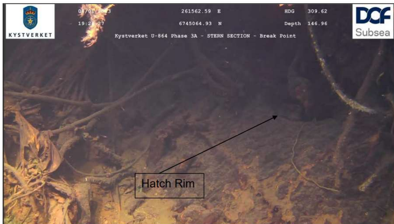
Figure 3.7 Interior watertight hatch, positively identifying the bulkhead
